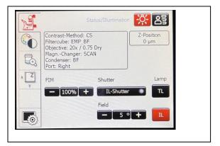
If by-eye fluorescence does not turn on: go to objective tab and press the "eye" button.
