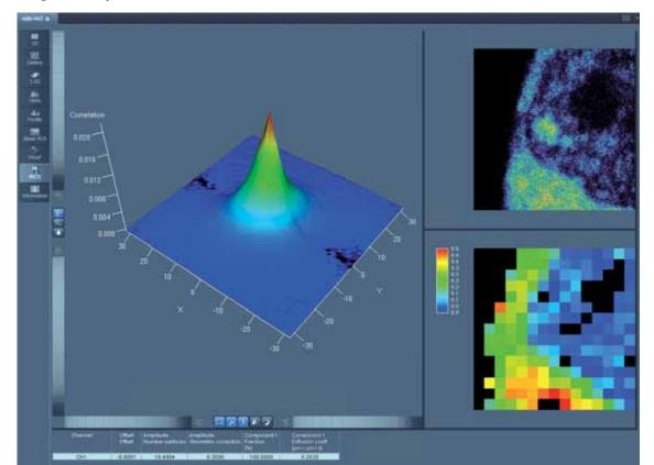
Color coded FLIM image (ps) of hepatocytes stained for Cytochrome C (Alexa 488) and Mirochondria (Alexa 564). Lifetime image acquired using 568 nm for excitation. Specimen: R. Pick and R. Nitschke; University of Freiburg, Germany
